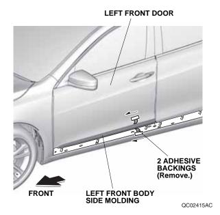
Using a rubber roller, apply firm pressure against the left front body side molding and roll from one end to the other. Apply firm pressure, especially at the ends.
