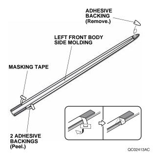
7. Align the left front body side molding with the template and attach it to the left front door as shown.
