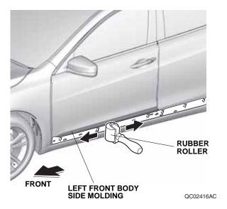
Peel back the adhesive backings, and tape them to the front surface of the left rear body side molding with the masking tape. Remove the small piece of adhesive backing.
