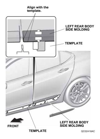
12. While applying light pressure against the molding, carefully remove the taped adhesive backings.
