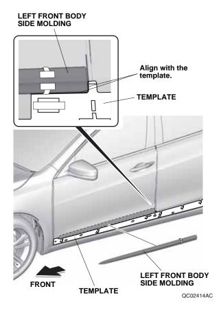
8. While applying light pressure against the left front body side molding, carefully remove the taped adhesive backings.
