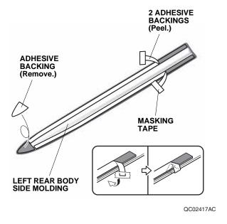
11. Align the left rear body side molding with the template and attach it to the left rear door as shown.
